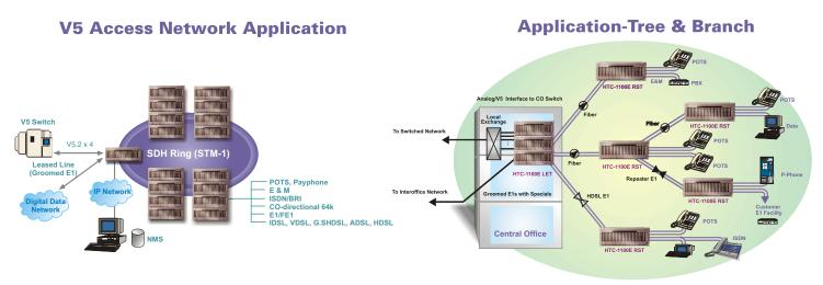
HTC-1100E is composed of a local exchange terminal (LET) connecting to one or more remote subscriber terminal(s) (RST). LET is usually located within a central office, while RSTs are located in customer areas to originate services. It not only utilizes various transport media but also can integrate into any network architecture. Universal, star, drop and insert, tree and branch, and SDH ring configurations are all supported by the flexible topologies of HTC-1100E.
