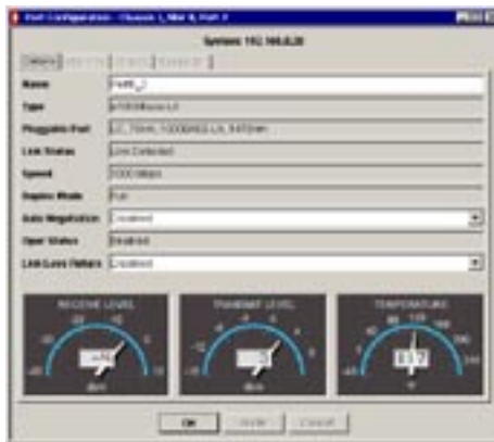
Quality of Optical Amplitude: Realtime measurement of the receive and transmit levels of the optical transceivers. Acts as integral power meter.
