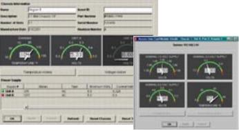
**Quality of Optical Amplitude:** Realtime measurement of the receive and transmit levels of the optical transceivers. Acts as integral power meter.
