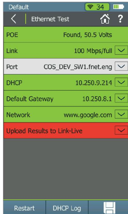
Figure 8: Ethernet Test UI.
