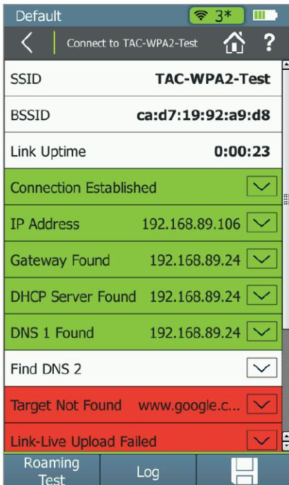
Figure 7: Connect to SSID UI.
